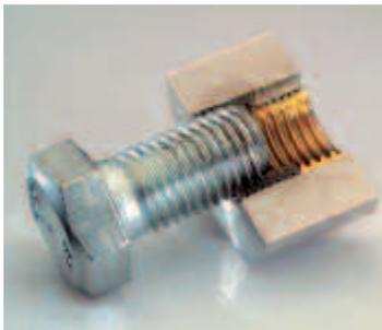
Ensats are self-tapping threaded inserts with external and internal thread, cutting slots or cutting bores. A continuous process of further development has brought about a number of major improvements to product characteristics. These inserts are protected by German and also foreign patents.
